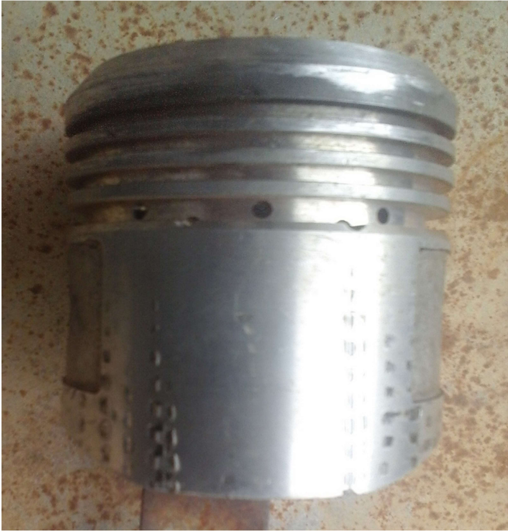
Plate 3.8. Modified Aluminium piston for test engine
