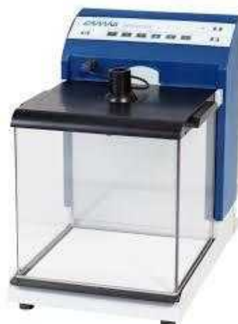
Effect directed analysis using Derivatiser
