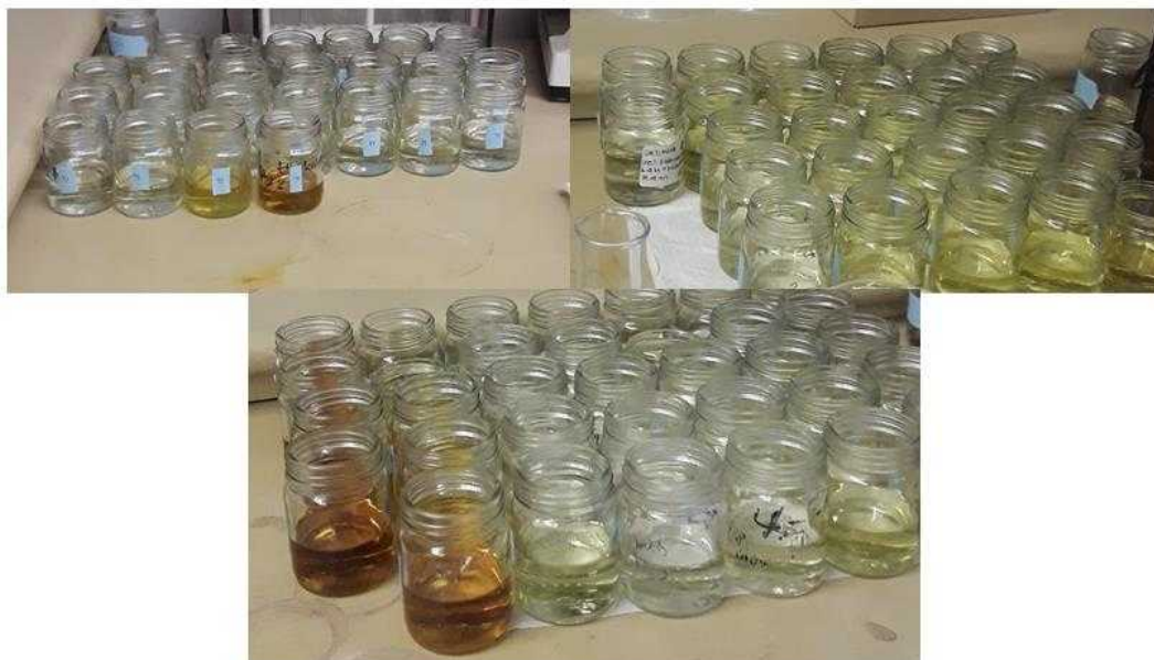
Figure 26: Picture of collected sub-fractions from the silica gel column of the EA fraction of Musa acuminata leaf
