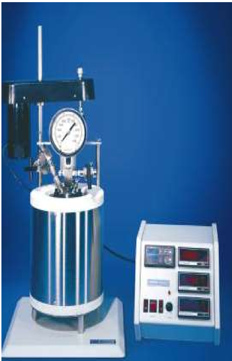
Figure 3.3: High Temperature/High Pressure Reactor, 500mL, with 4842 Temperature Controller
