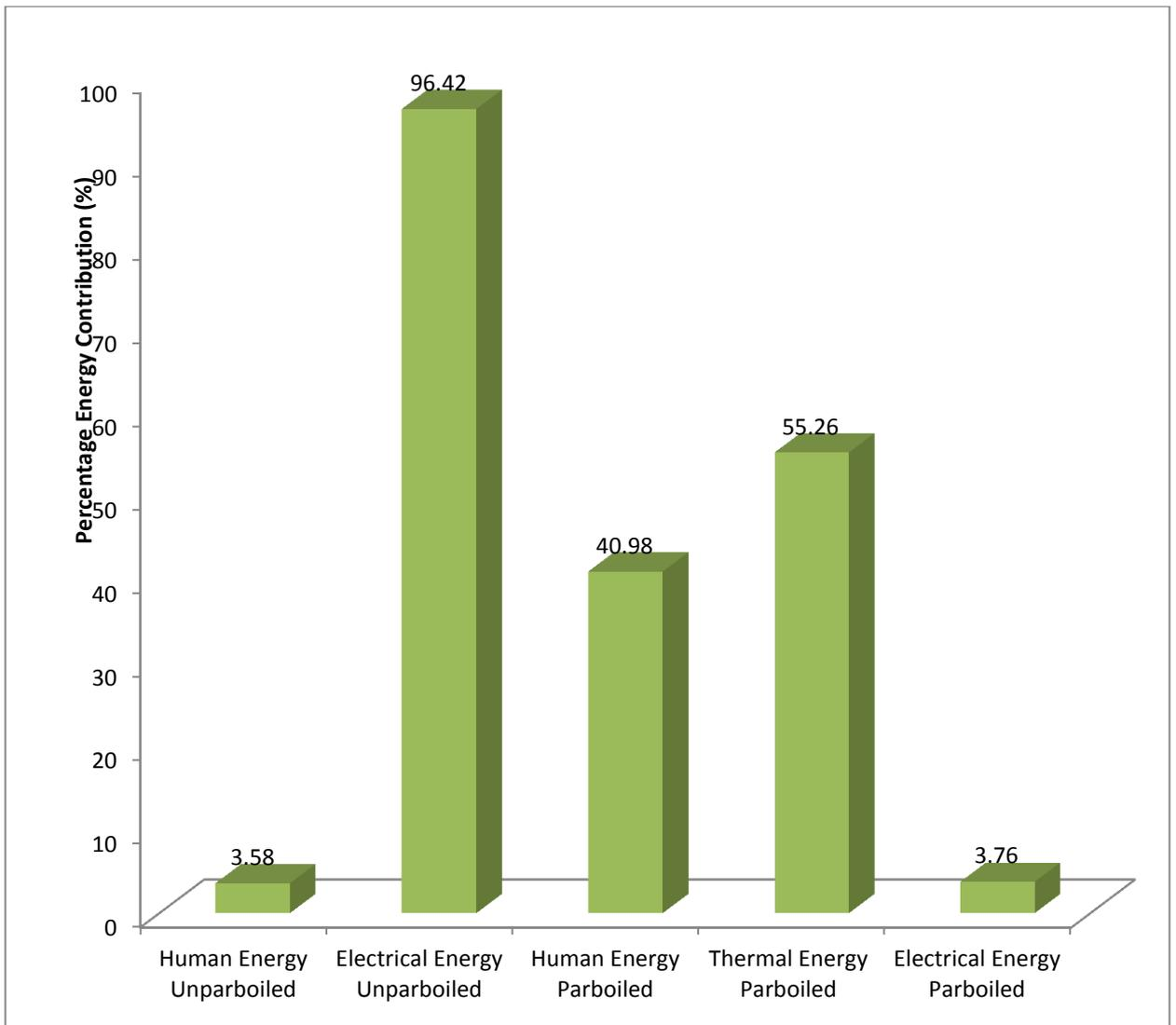
**Fig. 4.2. Forms of energy used during rice processing**
