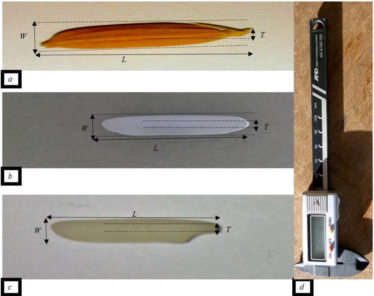
Plate 3.1. Paddy grain (a), White rice (b) and Parboiled polished rice (c) axial dimensions and digital vernier caliper (d)
