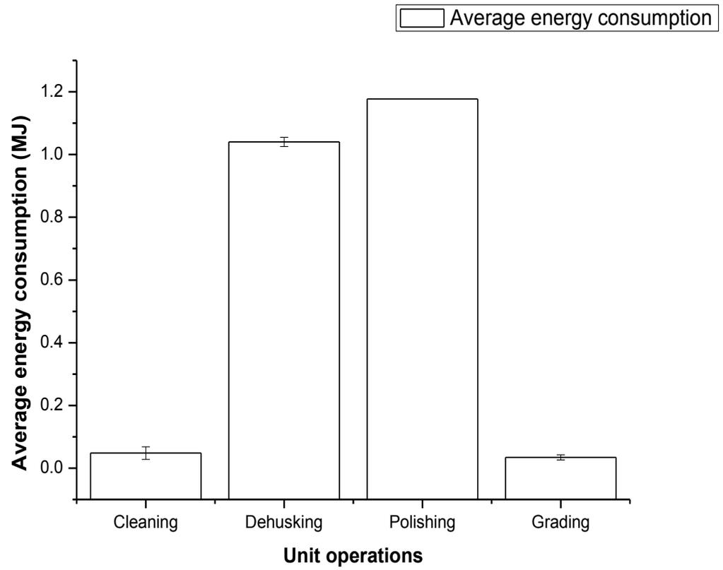
**Fig. 4.1. Average energy intensity pattern in processing paddy rice into white rice**
