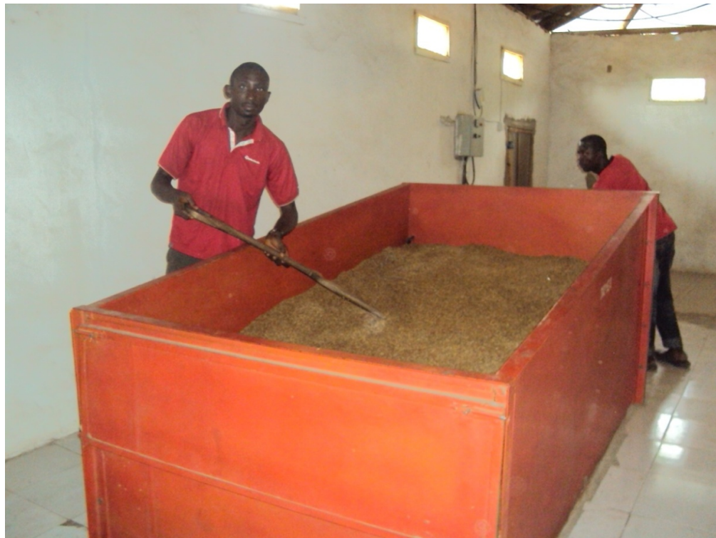
Appendix 2h: Rice Drying process by one ton per/batch dryer
