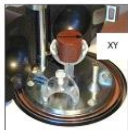
Fig. 3.9. Spinner magnetometer and its auto manipulations of six directions
