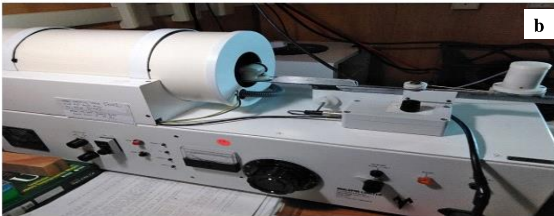
Fig. 3.7. (a) Thermal Demagnetizer MMTD80A with Eurotherm 3204 temperature controller and (b) shielded Molspin Alternating Field demagnetizer
