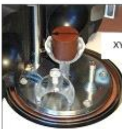
Fig. 3.9. Spinner magnetometer and its auto manipulations of six directions
