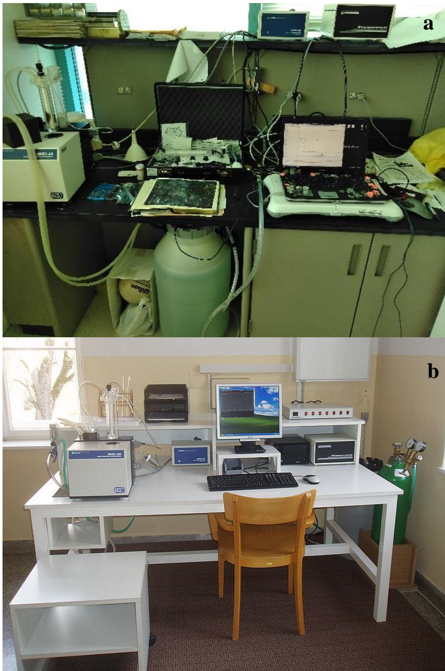
Fig.3.6. (a-b) multifunctional kappabridge (MFKI-FA) in Liquid Nitrogen and Argon gas environment
