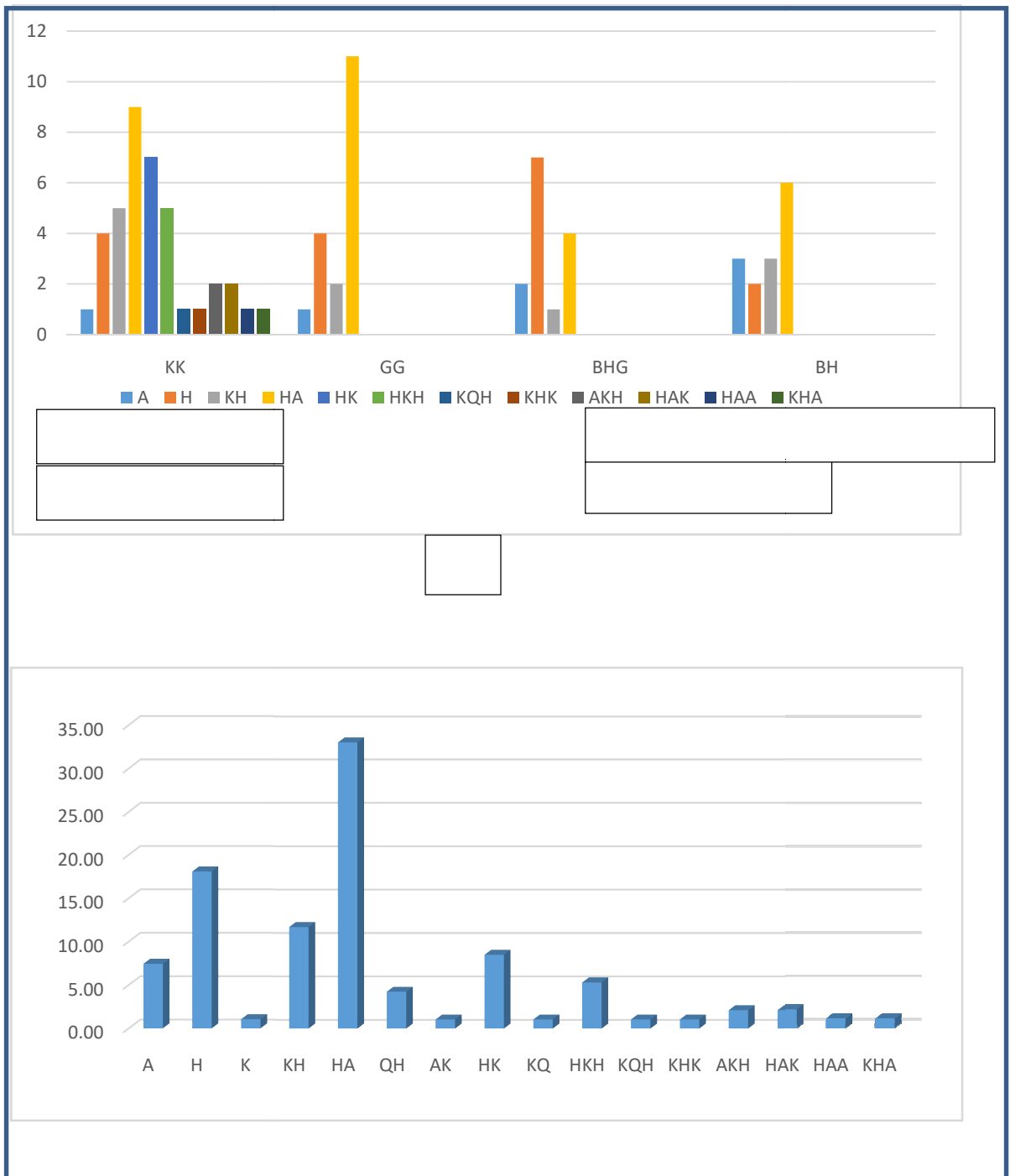
Fig. 4.13. (a) Distribution of the various type curves in the different rock units (b) Relative abundances of the different geo-electric field curves
