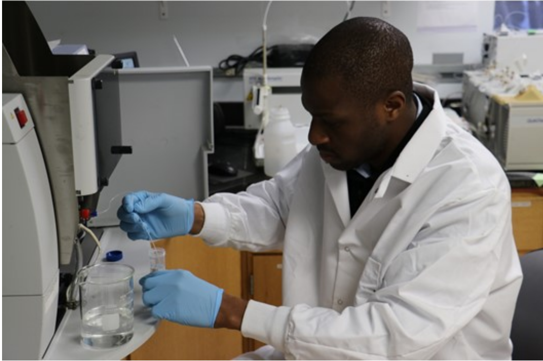
Plate 3.4. Measurement of concentration of cations in a sample using the nebulizing hose.
