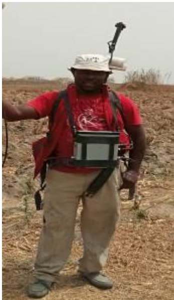
Setting up of the Magnetometer base station (b) Field data acquisition (operation) in the continuous (walkmag) mode (c) Field data acquisition in continuous mode
