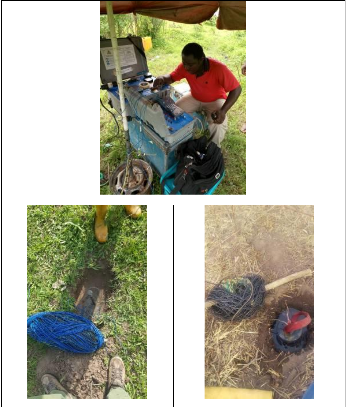
Field set up of the GDD 5000 Transmitter and 16C receiver; (b) Current injection electrode; and (c) Copper Sulphate Electrode Porous Pot
