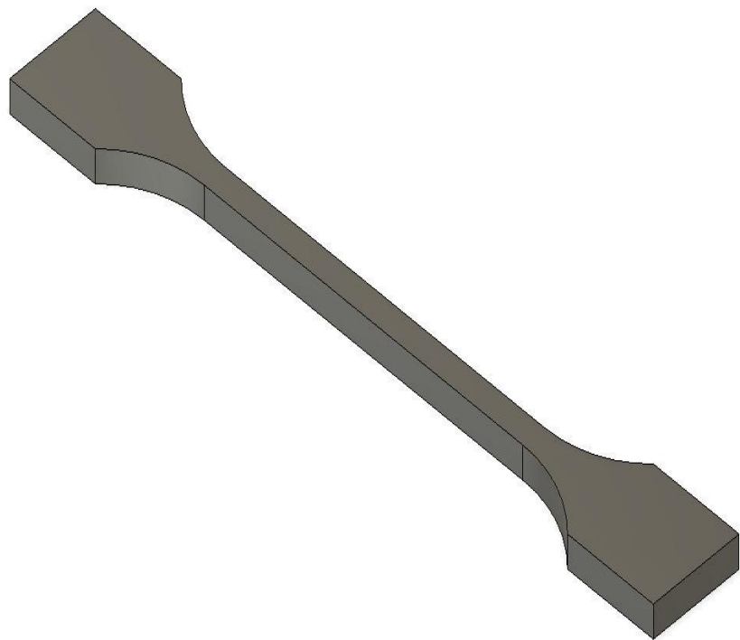
Fig. 3.2: Schematic illustration of the dog-bone shape tensile samples
