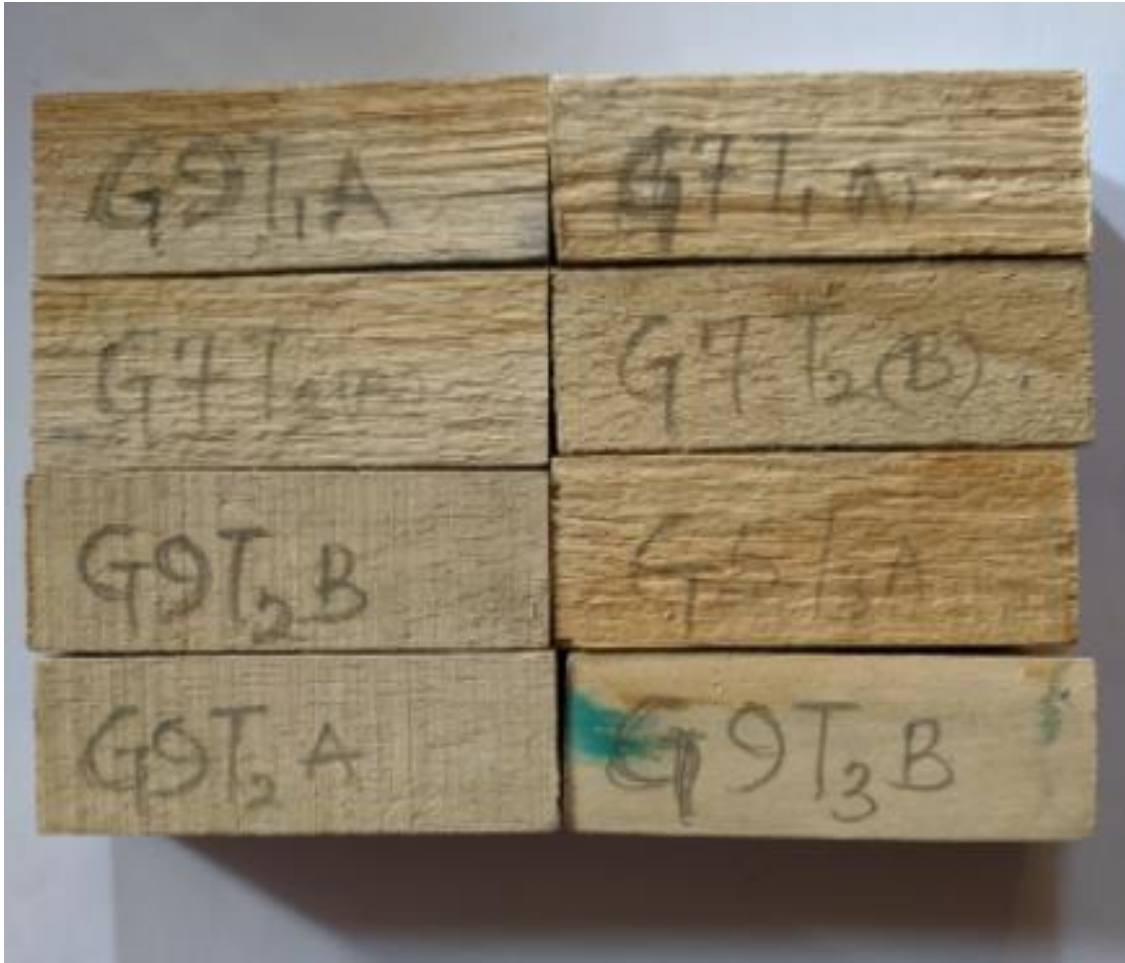
Plate 4.3: Colour changes in G. arborea wood samples bioincised with G. adpersum
