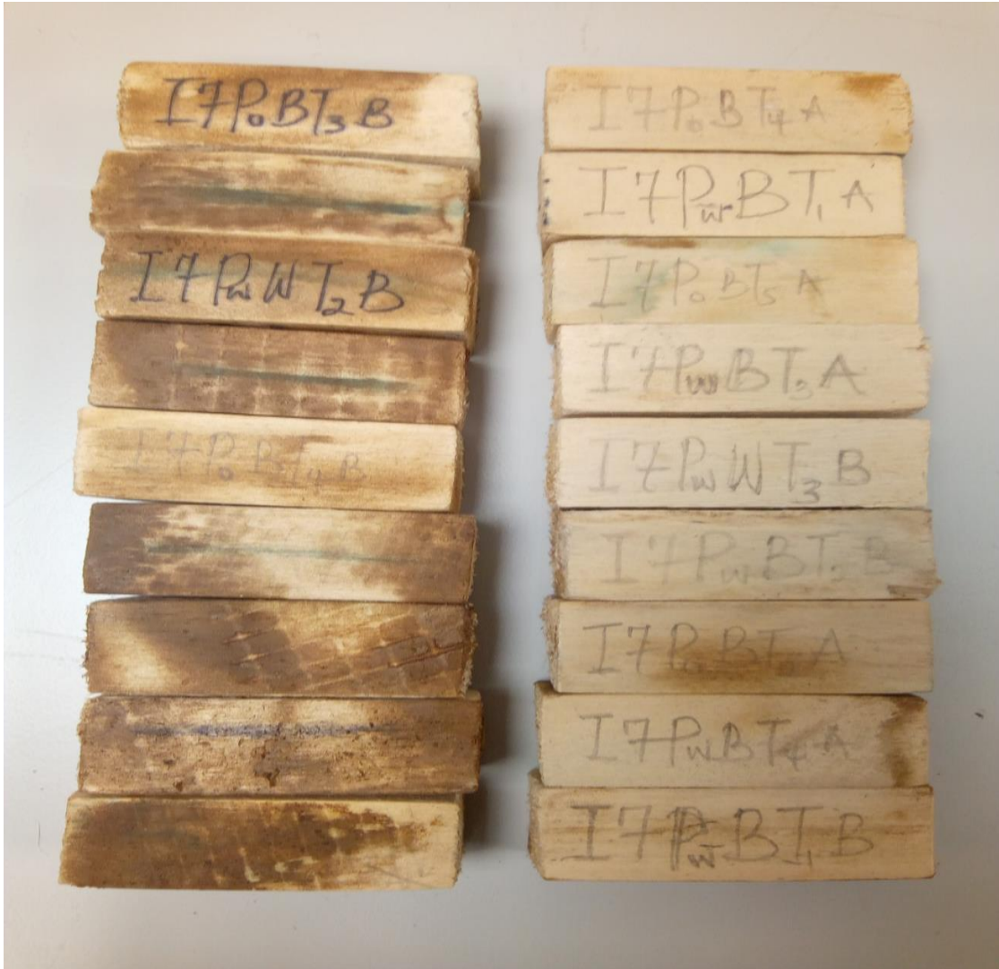
Plate 4.2: Colour changes in G. arborea wood samples bioincised with I. dryophilus
