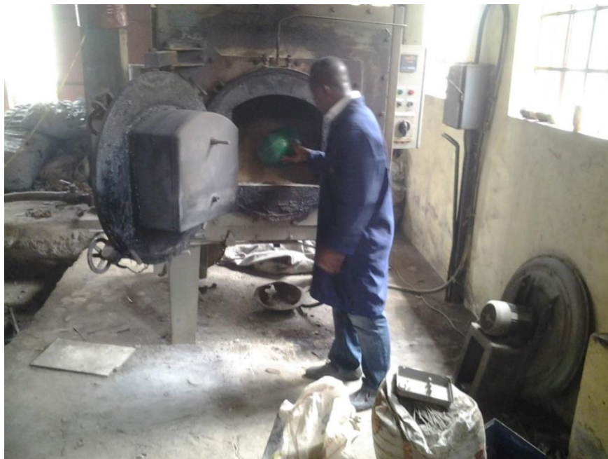
Plate 3.1: Rice Husk in production using the closed furnace.
