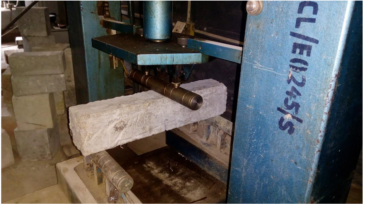
Plate 3.4: Three-point bending test
