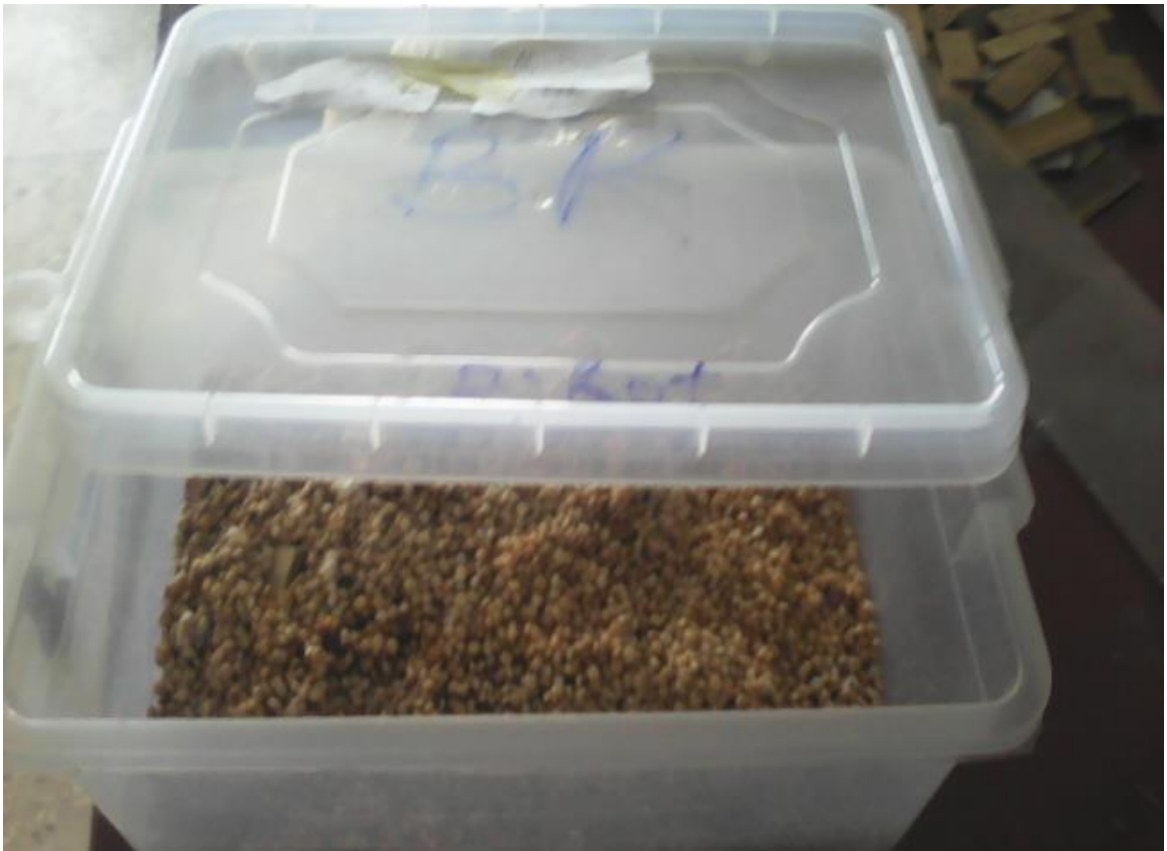
Plate 3.18: Inoculated Bamboo samples in the inoculation box
