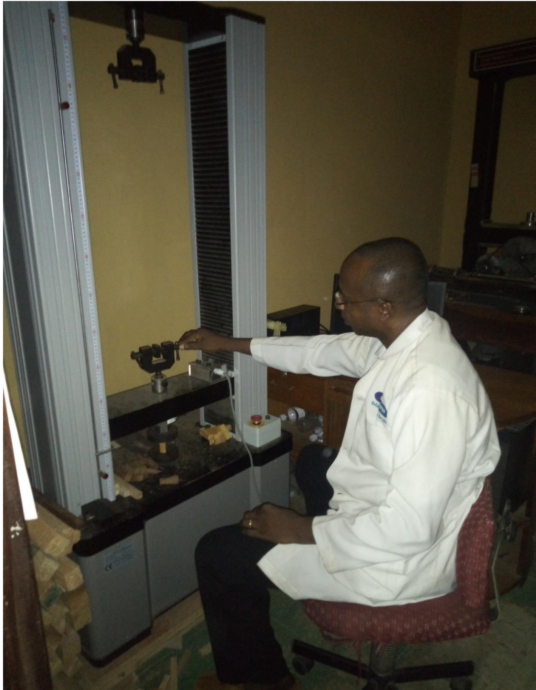
Plate 3.26: Shear Strength Parallel to Grain test of samples on Universal Testing Machine
