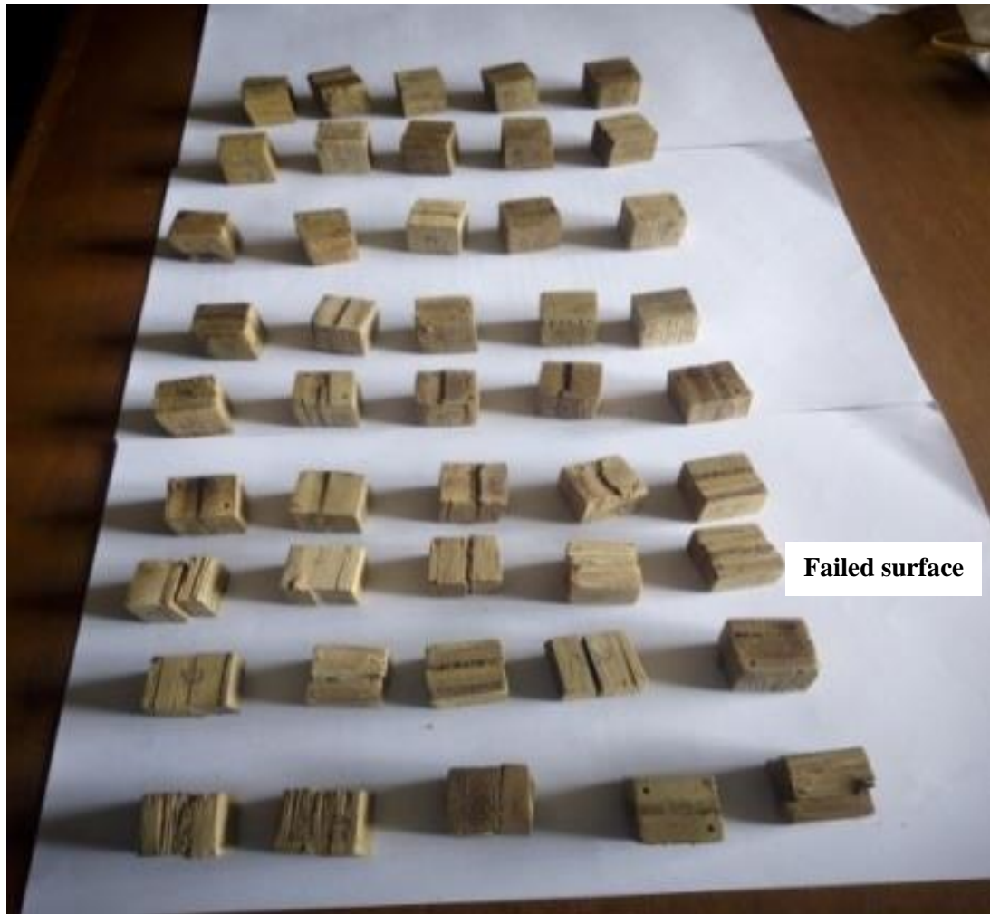
Plate 3.27: Failed laminated bamboo samples after shear test
