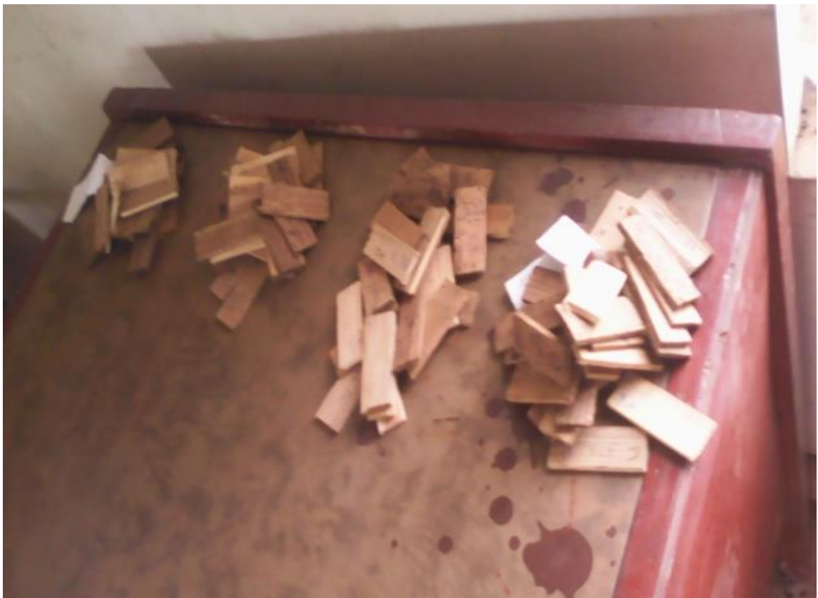
Plate 3.14: Bamboo samples being prepared for fungal (white or brown rot) inoculation
