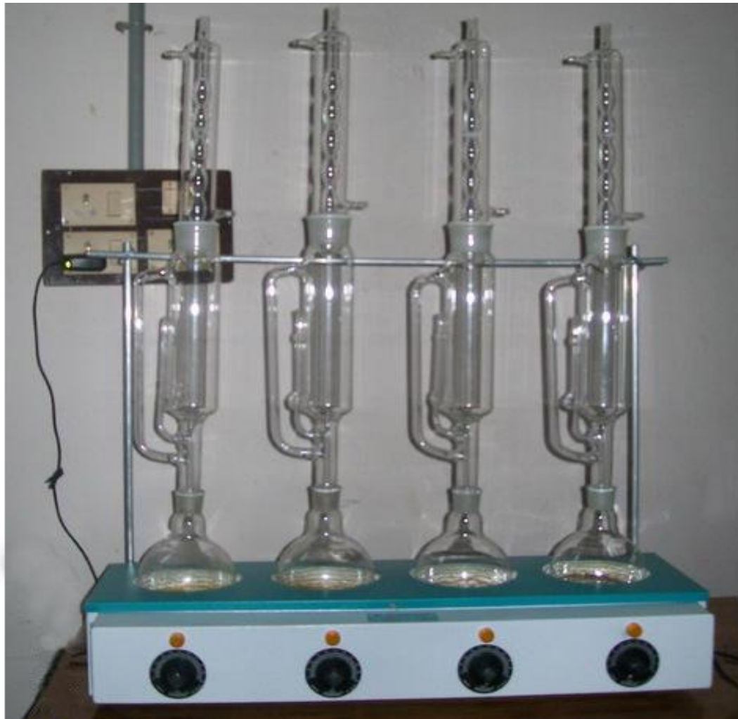
Plate 3.5: A complete set of multiple Soxhlet Extractor Apparatus
