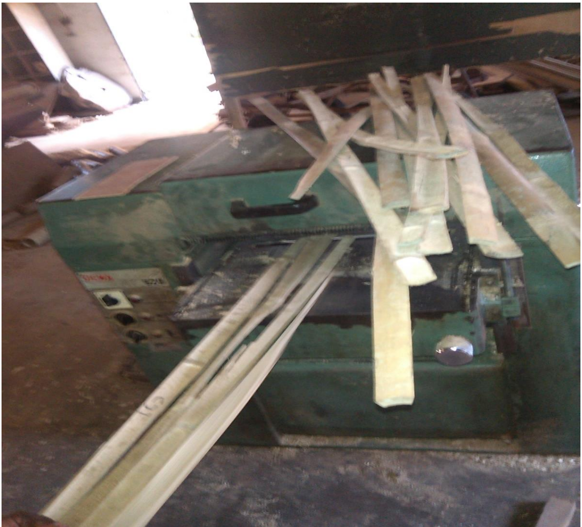
Plate 3.23: Prepared bamboo strips with the thickening machine
