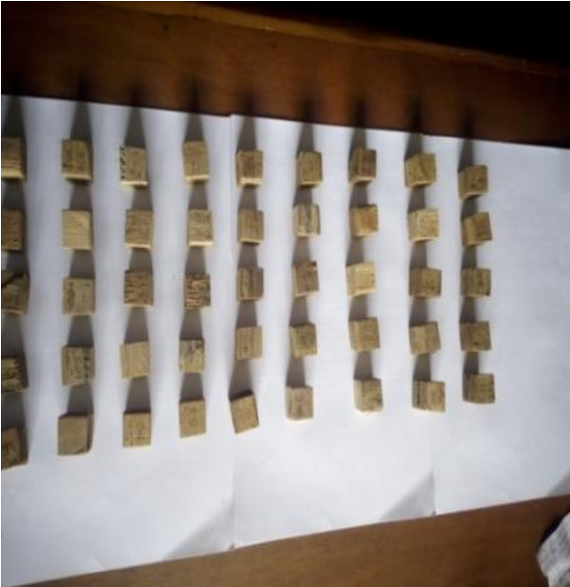
Plate 3.25: Shear strength samples processed from laminated bamboo boards
