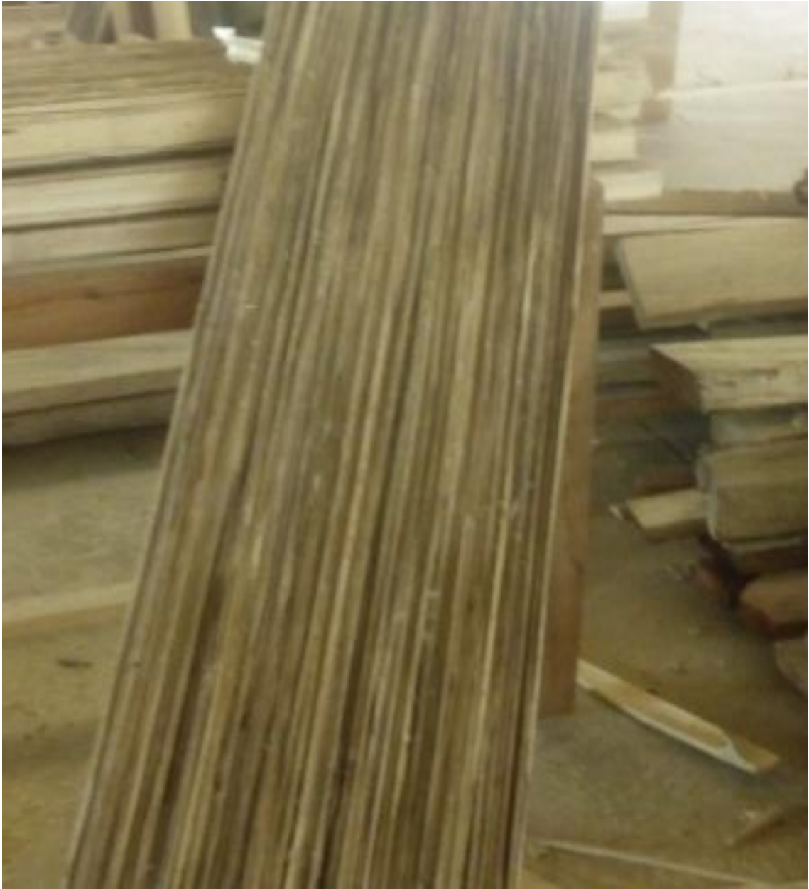
Plate 3.24: Laminated bamboo strips using top bond glue as binder
