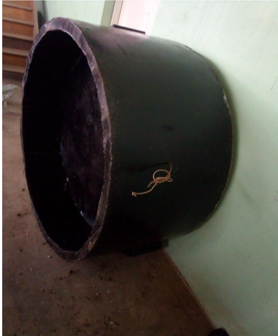
Plate 10.1: The Bottom of the Frying Pan Showing the Outlet of the Heat Resistant Cable that Connects the Electrical Filament to the Distribution Cabinet
