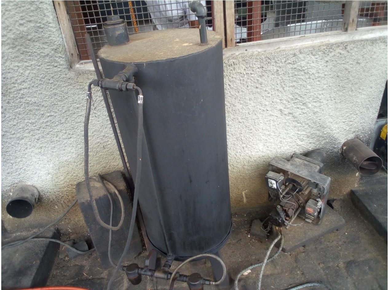
Plate 10.2: One of the Diesel Tanks for the Mechanized Fryer and a Burner that was broken down during a Frying Operation
