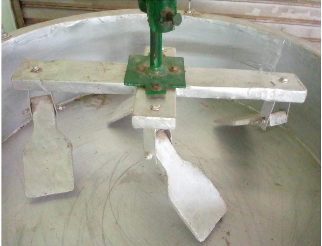
Plate 4.5: Frying Mechanism of the Fryer
