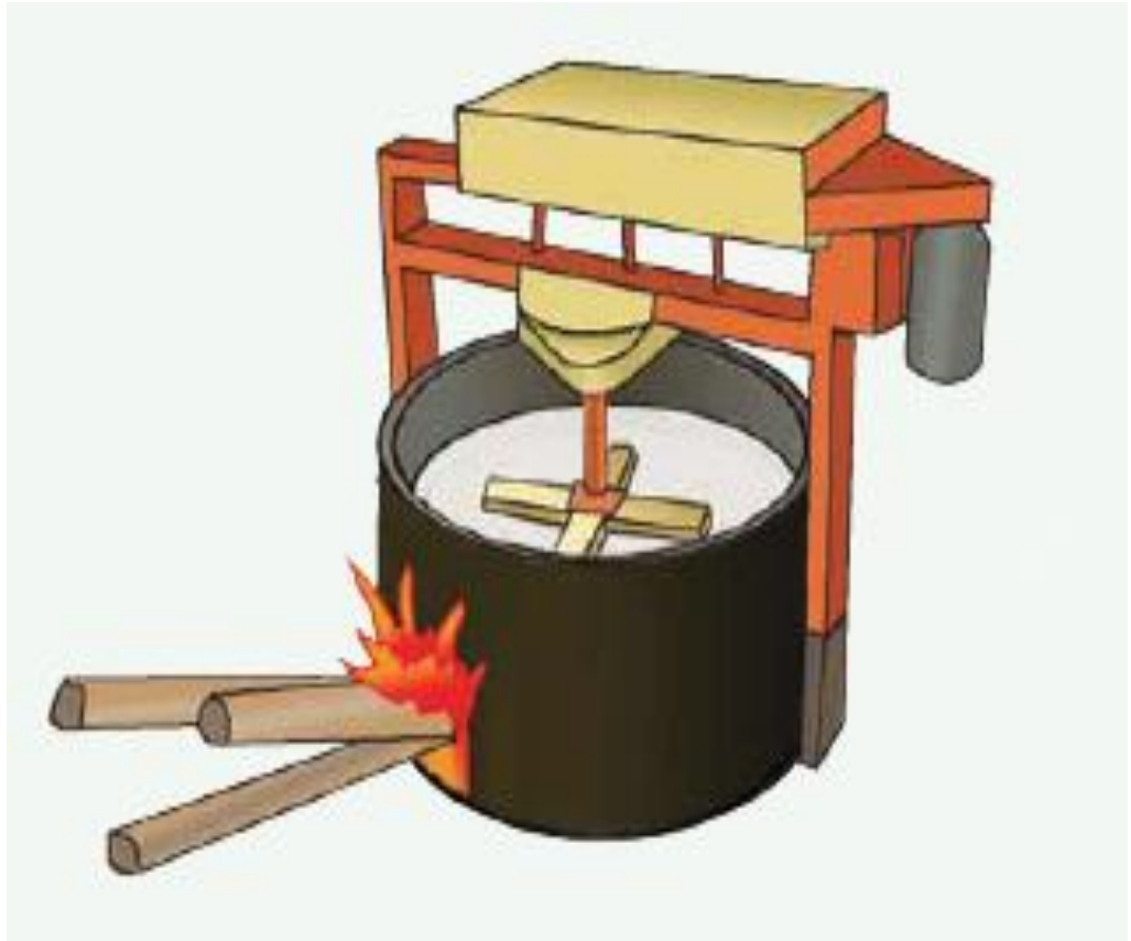
Plate 2.11a: Mechanical Gaari Fryer Back View (Using Fire Wood as Heat Source)
