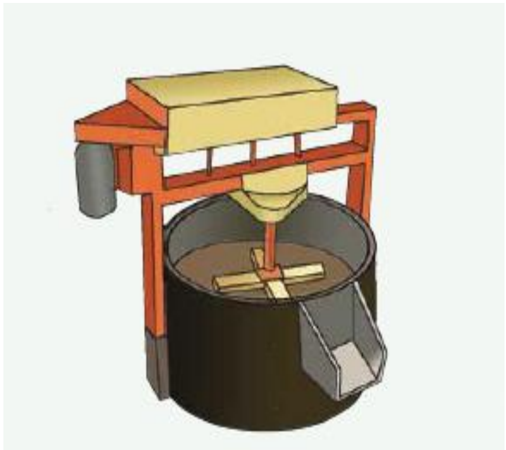
Plate 2.11b: Mechanical Gaari Fryer Front View
