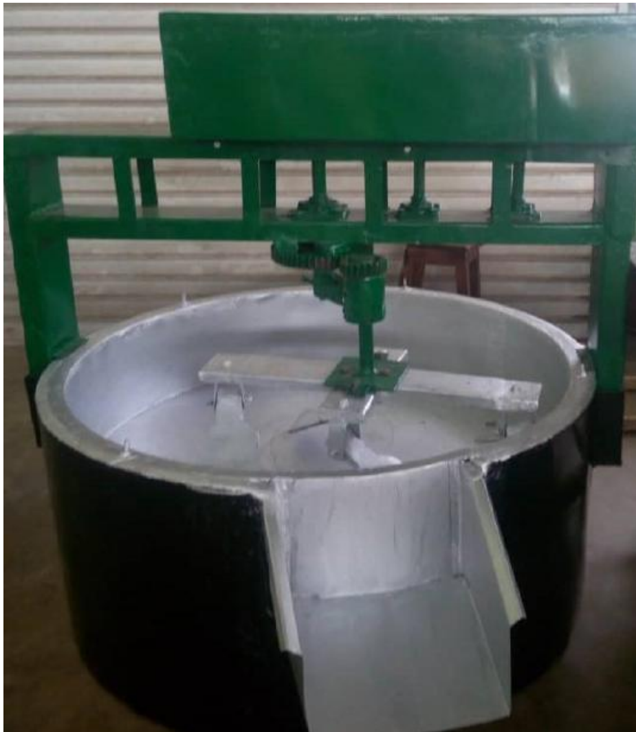
Plate 4.1: The Automated Gaari Frying Machine
