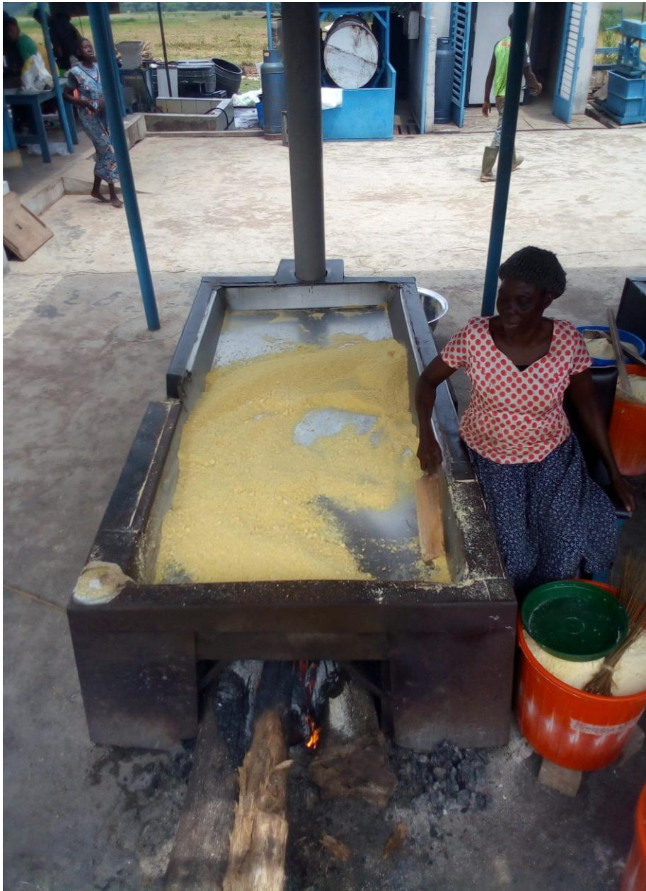
Plate 10.4: Manual Garri Frying Operation
