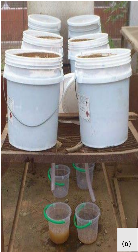
Plate 3.1: Lysimeters and drainage collection facilities (a), and okra plant in a lysimeter at 5 WAS (b)
